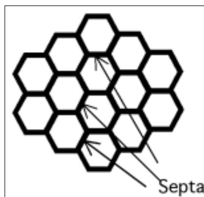
**Figure 13:** Transverse view of a parallel hole collimator with hexagonal openings.
